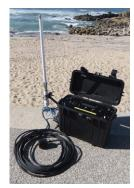
The Communications Gateway is a hub that supports wireless and acoustic communication to the LAUV. It allows multiple operators to control and monitor multiple vehicles in a networked environment over distinct platforms, including Android smart phones. The device is battery powered for full autonomy and portability. It comes in a rugged waterproof enclosure that allows installation in a buoy, if required.
